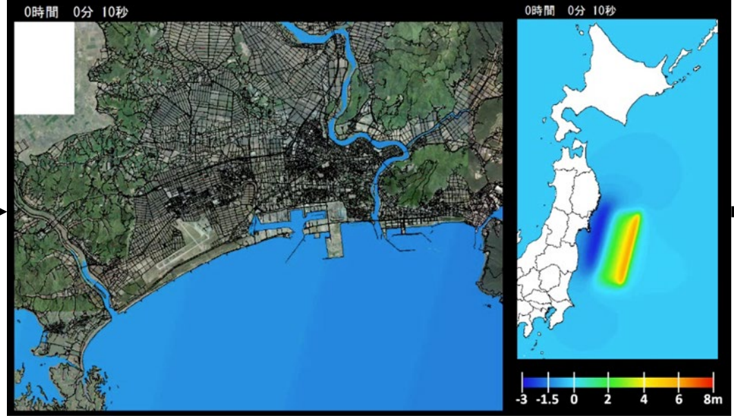
Real-time simulation on Supercomputer AOBAs at Tohoku University with considering current costal facilities and tide height at the occurrence.
