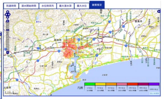
Real-time simulation on Supercomputer AOBAs at Tohoku University with considering current costal facilities and tide height at the occurrence.
