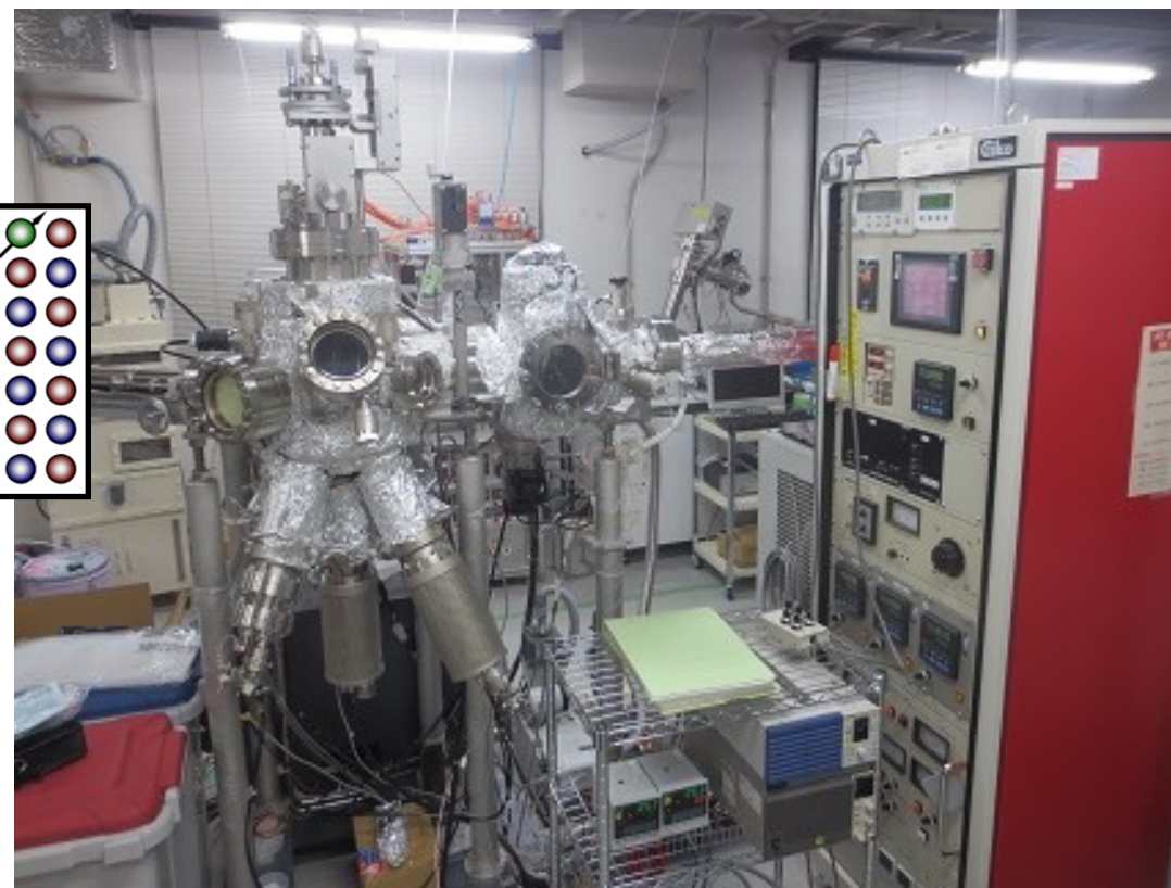
A molecular beam epitaxy system (Hamaya Group in Osaka Univ)
